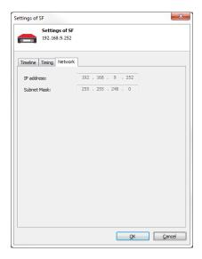
Network settings for a MYLAPS X2 Decoder cannot be changed in this Dialog: Settings can be changed via the X2 Utility or X2 Manager.
