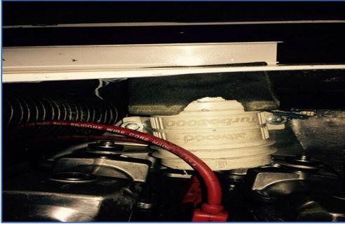
**Figure 2a** Fan & opening covers #3 & #4 cylinders only.
